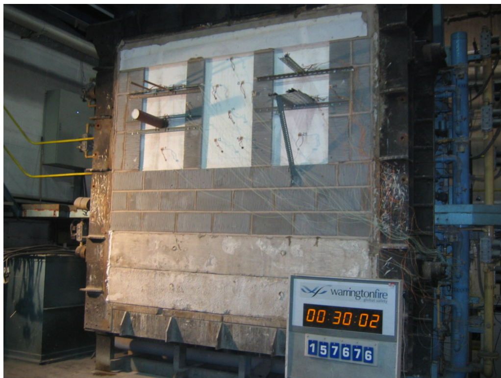
The unexposed face of the assembly after 30 minutes of testing
