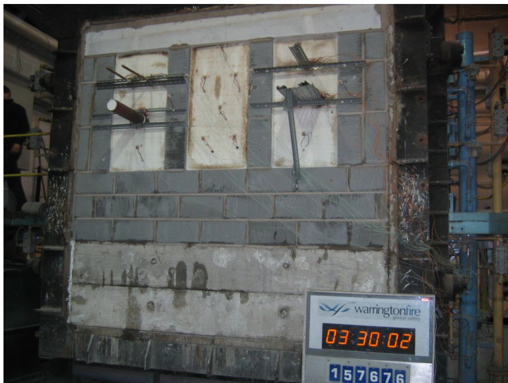
The unexposed face of the assembly after 210 minutes of testing
