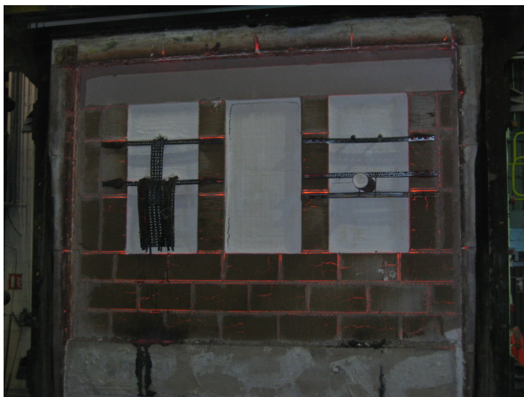
The exposed face of the assembly immediately after the test
