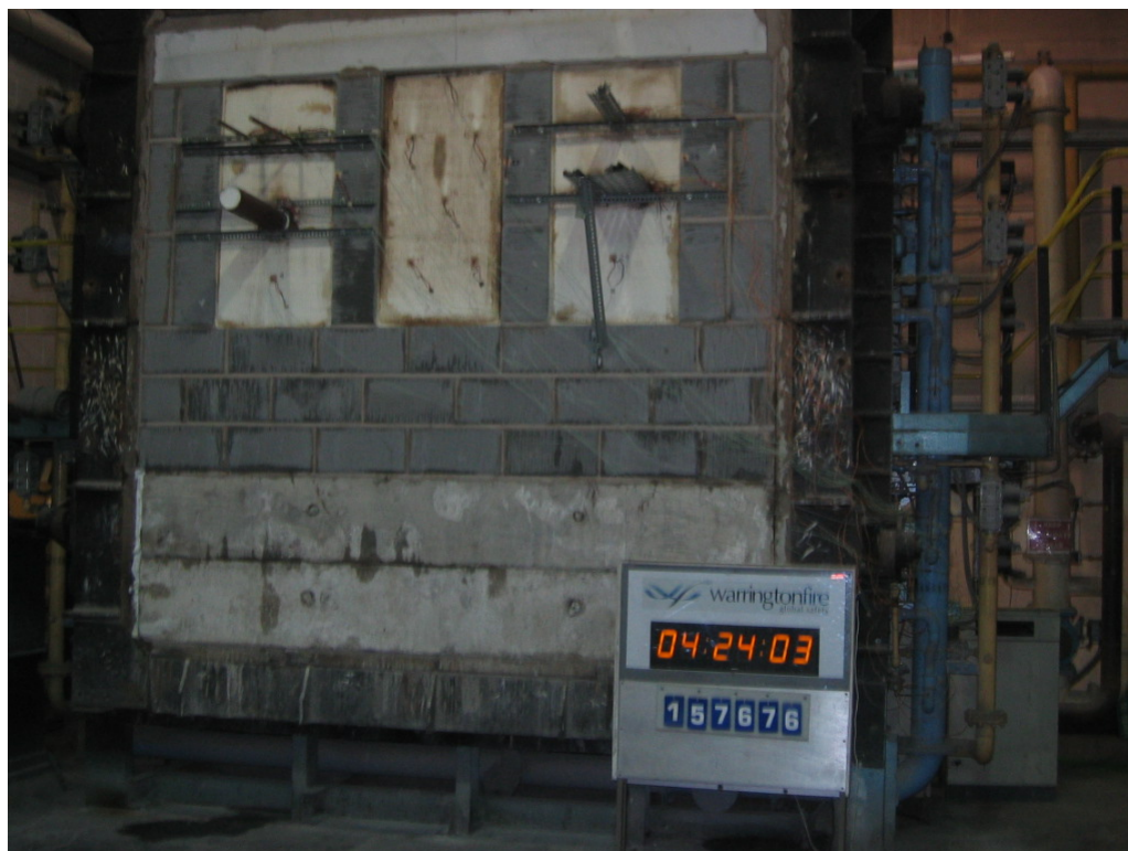
The unexposed face of the assembly after 264 minutes of testing
