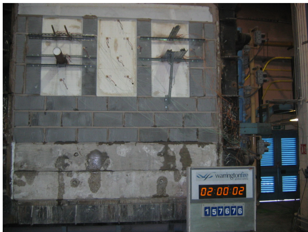
The unexposed face of the assembly after 120 minutes of testing
