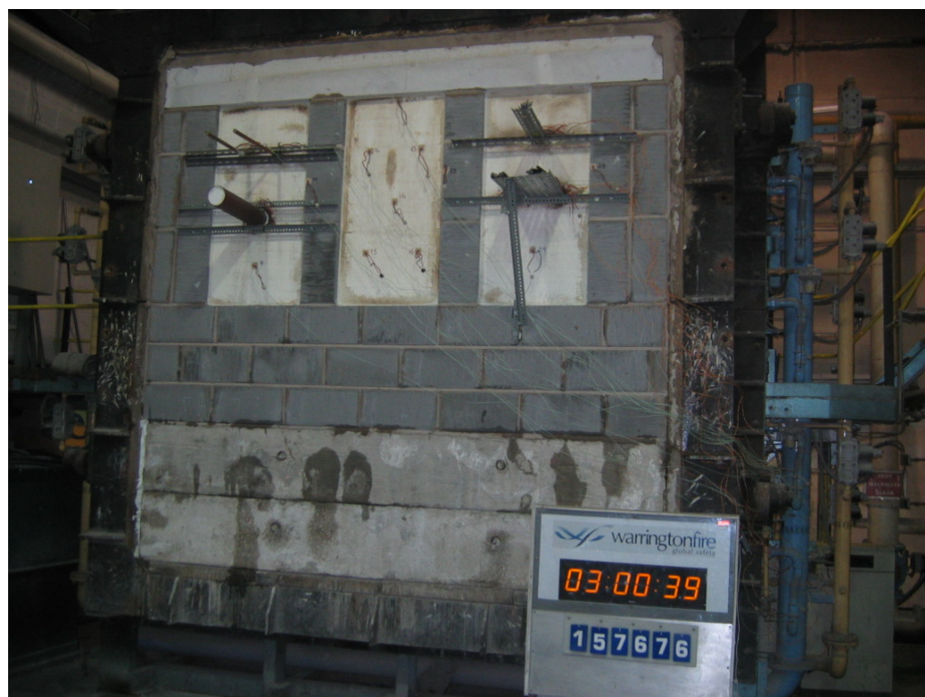
The unexposed face of the assembly after 180 minutes of testing
