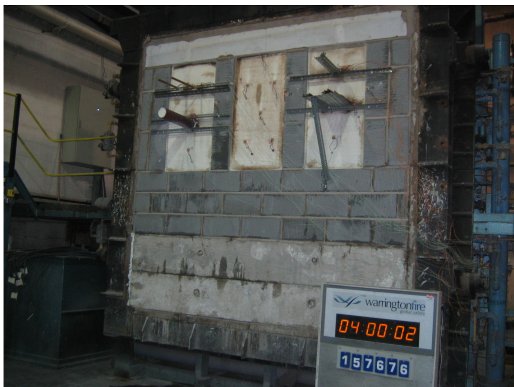
The unexposed face of the assembly after 240 minutes of testing
