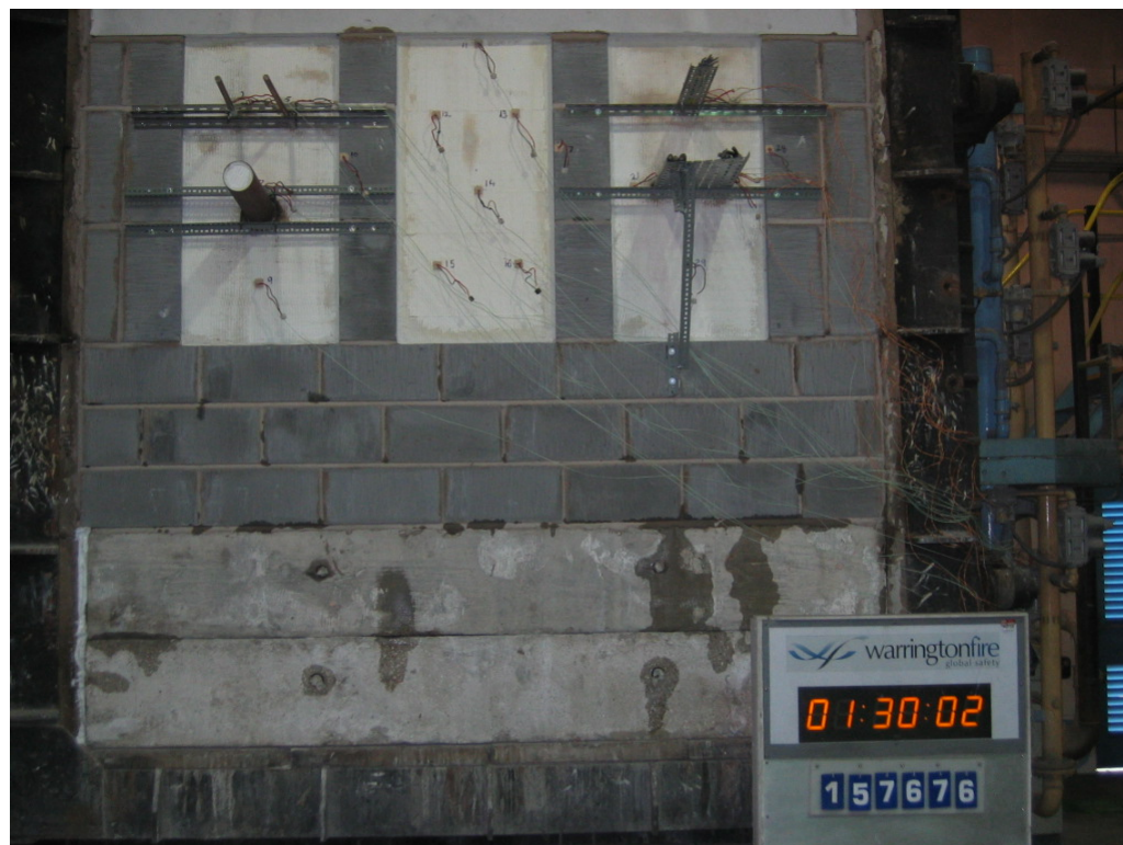
The unexposed face of the doorsets after 90 minutes of testing
