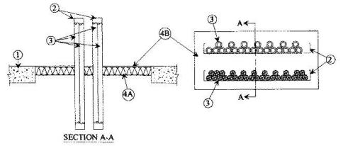
1. Floor or Wall Assembly — Min 4-1/2 in. thick reinforced lightweight or normal weight (100<u>150</u> pcf) concrete. Wall may also be constructed of any UL Classified **Concrete Blocks**<sup>\*</sup>. Max area of opening is 960 sq in. with max dimension of 40 in. See **Concrete Blocks** (CAZT) category in the Fire Resistance Directory for names of manufacturers.
