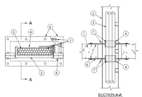
1. **Floor or Wall Assembly** — Min 4-1/2 in. (114 mm) thick lightweight or normal weight (100<u>150</u> pcf or 1600-2400 kg/m>) concrete. Wall may also be constructed of any UL Classified **Concrete Blocks\*.** Max area of opening <u>900</u> sq in. (5806 cm<sup>2</sup>) with max dimension of 30 in. (762 mm).
