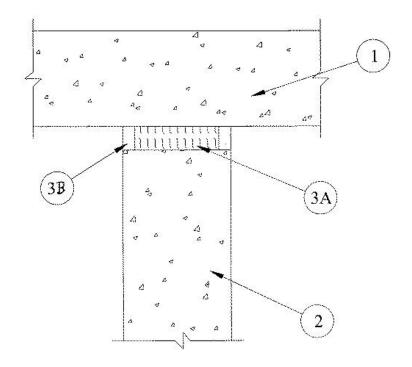
1. Floor Assembly — Precast Autoclaved Aerated Concrete\* — Min 4 in. thick as specified in Design No. K909, K910, P932 or P933 in the UL Fire Resistance Directory.
