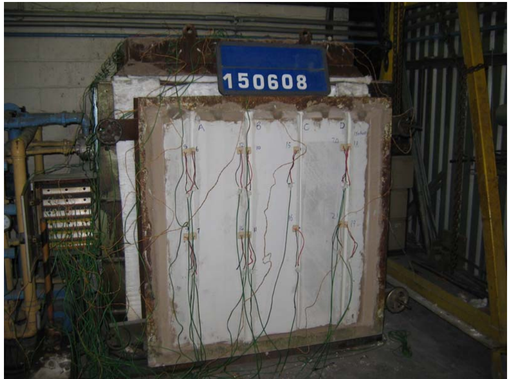
The unexposed face of the wall construction prior to testing
