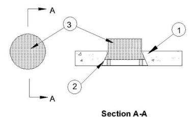
1. **Floor Assembly** — Min 2-1/2 in. (64 mm) thick reinforced lightweight or normal weight (100-<u>150</u> pcf or 1600-2400 kg/m<sup>3</sup>) concrete.
