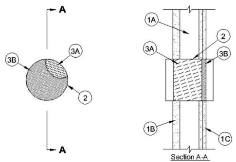
1. **Wall Assembly** — The 1 or 2 hr fire-rated gypsum board/stud shaft wall assembly shall be constructed of the materials and in the manner specified in the individual U400 Series Wall and Partition Designs in the UL Fire Resistance Directory and shall incorporate the following construction features:
