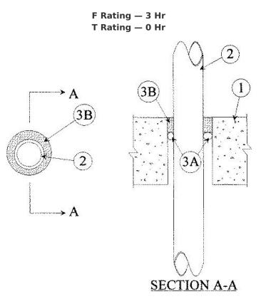
1. **Floor or Wall Assembly** — Min 4-1/2 in. thick reinforced lightweight or normal weight (100-<u>150</u> pcf) concrete. Wall may also be constructed of any UL Classified **Concrete Blocks\*.** Max diam of opening is 6 in. See **Concrete Blocks** (CAZT) category in the Fire Resistance Directory for names of manufacturers.
