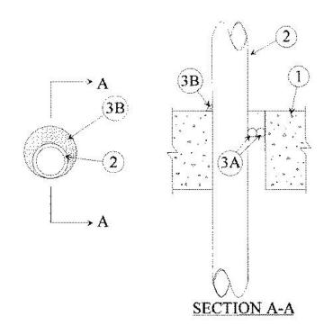
1. **Floor or Wall Assembly** — Min 4-1/2 in. thick reinforced lightweight or normal weight (100-<u>150</u> pcf) concrete. Wall may also be constructed of any UL Classified **Concrete Blocks\*.** Max diam of opening is 4 in. See **Concrete Blocks** (CAZT) category in the Fire Resistance Directory for names of manufacturers.
