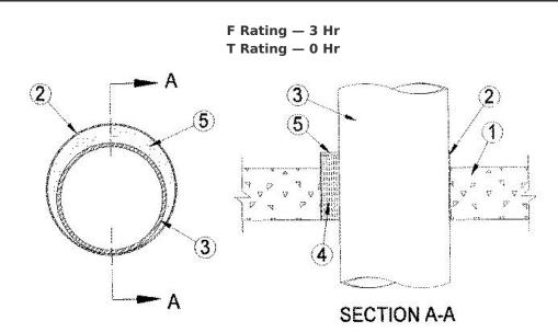
1. **Floor or Wall Assembly** — Min 4-1/2 in. thick reinforced lightweight or normal weight (100-<u>150</u> pcf) concrete. Wall may also be constructed of any UL Classified **Concrete Blocks\*.** See **Concrete Blocks** (CAZT) category for names of manufacturers.
