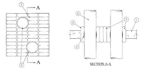
1. **Floor or Wall Assembly** — Min 4-1/2 in. thick reinforced lightweight or normal weight (100-<u>150</u> pcf) concrete. Wall may also be constructed of any UL Classified **Concrete Blocks\*.** Max are of opening not to exceed 576 sq. in. with a max dimensions of 24 in.
