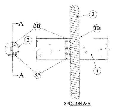
1. **Floor or Wall Assembly** — Min 4-1/2 in. thick reinforced lightweight or normal weight (100-<u>150</u> pcf) concrete. Wall may also be constructed of any UL Classified **Concrete Blocks\*.** Max diam of opening is 3 in.
