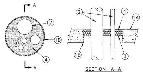
1A. **Floor or Wall Assembly** — Min 2-1/2 in (64 mm) thick floor or 3 in. (76 mm) thick wall of reinforced light weight or normal weight (100-<u>150</u> pcf or 1600-2400 kg/m³) concrete. Wall may also be constructed of any UL Classified**Concrete Blocks**\*. Max diam of opening is 15-1/4 in. (387 mm).
