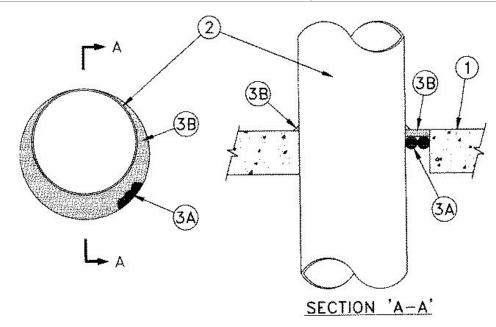
1. Floor or Wall Assembly — Min 2-1/2 in. (64 mm) thick reinforced light weight or normal weight (100<u>150</u> pcf or 1600-2400 kg/m<sup>3</sup>) concrete. Floor may also be constructed of any 6 in. thick UL Classified hollow-core**Precast Concrete Units**\*. Wall may also be constructed of any UL Classified **Concrete Blocks**\*. Max diam of opening is 24-7/8 in. (632 mm). When precast concrete units are used the max diam of opening is 7 in. (178 mm).
