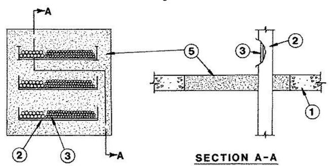
1. **Floor or Wall Assembly** — Min 2-1/2 in. thick reinforced lightweight or normal weight (100-150 pcf) concrete. Wall may also be constructed of any UL Classified **Concrete Blocks\*.** Max area of opening is 1024 sq in. with max dimension of 32 in.
